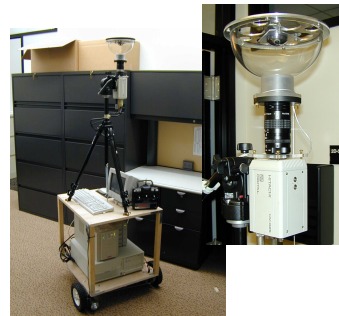
Figure 4. Omnidirectional Camera Setup. The motorized cart contains the camera, frame grabber, RAID disks, and battery.
