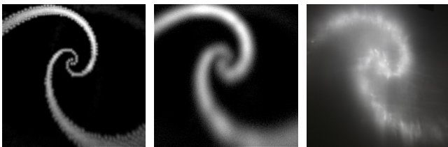
Figure 5: Left: Simulated reflectance off the material against a wall, using a point-light source and assuming a near mirror-like base BRDF. Center and Right: Verification of the simulation by simulating a more realistic base BRDF (center) to match a photograph of a reflection from a physical sample (right).
