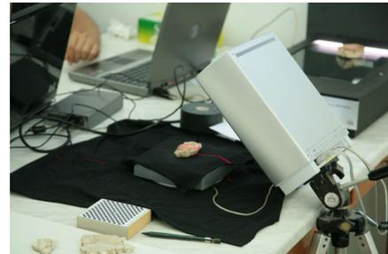
Figure 4.3: Using an off-the-shelf 3-D scanner (front), positioned at a 45-degree angle relative to a motorized turntable, we can acquire the front, back, and sides of a fragment with a single manual flip. A 2-D scanner (rear) simultaneously acquires high-resolution color and normals.
