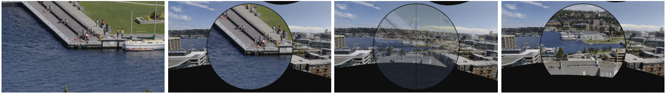
Figure 1: We explore four modes for panning high-resolution panoramas in virtual reality devices. Left to right: normal mode, circle mode, transparent circle mode, and zoom circle mode. The latter two provided equally successful interfaces.
