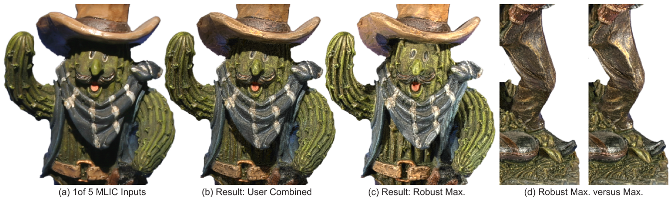
Figure 7: The user selected the input image (a) as the only base image to generate the result in (b). While the overall lighting of (a) is preserved, the image is enhanced by detail from all the other MLIC images. In (c) the robust maximum is used to construct the base image. Shadows are minimal making the image appear a bit flatter; but detail is revealed everywhere. In (d) the robust maximum attenuates the specular highlights on the upper leg of this metallic object, while the true maximum accentuates these highlights.
