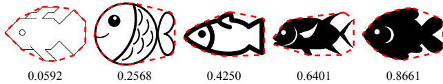
Figure 4: Five fish pictograms enclosed by their convex hulls (red dashed polylines), and the resulting blackness values.
