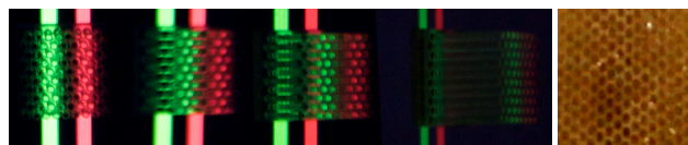
Fig. 4. Air cladding fibers have 180 degree field of view and excellent transmission, but they are impractical since support material is added between the fibers during printing. This support material is very hard to clean for the intricate fiber geometries used in this work. From left to right, we see light imaged from increasingly grazing angles. On the back, a laptop screen feeds light into the bundle. At extreme right, we show the hexagonal cross-section at the base of our fibers. This shape improves tiling of the input image plane with no observable loss in fiber transmission.
