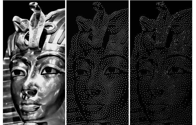
Figure 8: Part of the image used to create the stippling (left). Point set (center). Image of the stippling facricated with a 3D printer (right).
