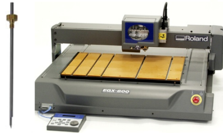
Figure 10: We used a Roland EGX-600 engraver for our experiments. This is a 3-degree-of-freedom milling machine with high-precision axes and a fine-tipped cutter (as shown in closeup at left).
