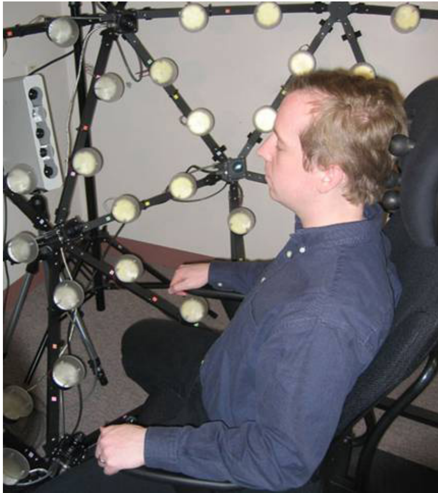
Figure 3.8: Acquisition setup designed for measuring the reflectance properties of human skin [112].
