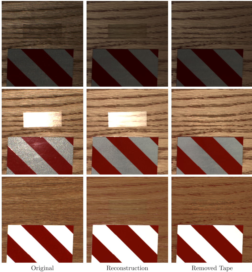
Figure 4.14: The Wood-Tape dataset consists of a piece of oak partially covered by semi-transparent tape and retroreflective bicycle tape. Left: Three original images illustrate that the tape disappears for some incident and reflected directions, making this a challenging dataset to separate into its component materials. Also note the significant brightening of the lower image due to retroreflection. Middle: Reconstruction provided by a shade tree with five terms, computed using the ACLS algorithm. Right: We edit the weight maps to remove the tape. Although our separation was not perfect, the resulting edits display few artifacts.
