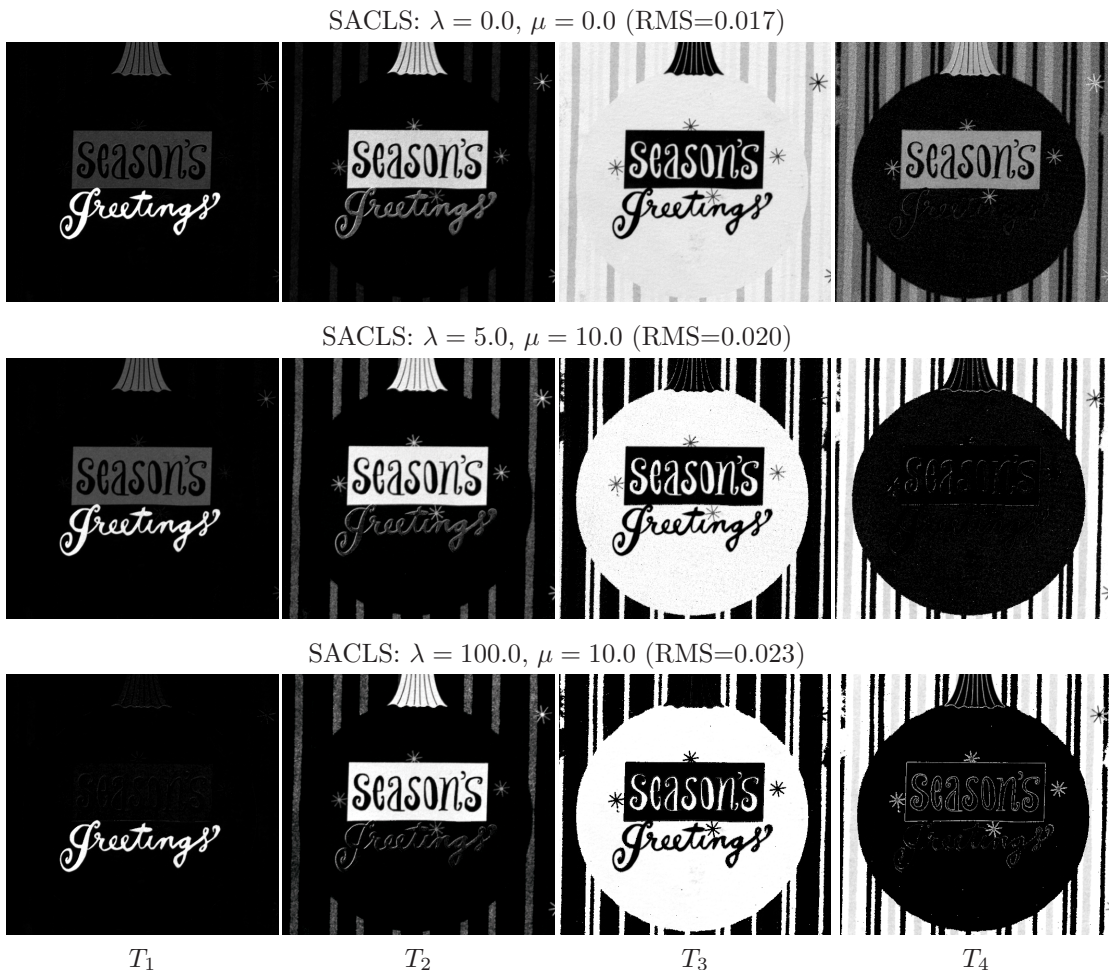
Figure 4.6: The blending weights computed from the “Season’s Greetings” dataset using SACLS with different settings of \lambda and \mu . Increasing values of \lambda force the algorithm to behave more like clustering, trading reconstruction accuracy for a more meaningful separation. RMS errors refer directly to the quality of reconstruction, without taking into account the additional error terms for sparsity or other constraints.
